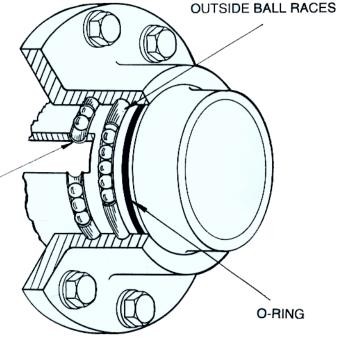
**REPLACEMENT SEALS**, developed by Gammon specifically for Chiksan® FMC swivels, overcome "weeping" or dripping when the system is not pressurized. Instead of a molded ring, our seal system uses 2 Viton o-rings that seal at both low and high pressures. A perfectly machined o-ring carrier ring is supplied in the kit for initial installation. Thereafter, only the o-rings need to be replaced.
