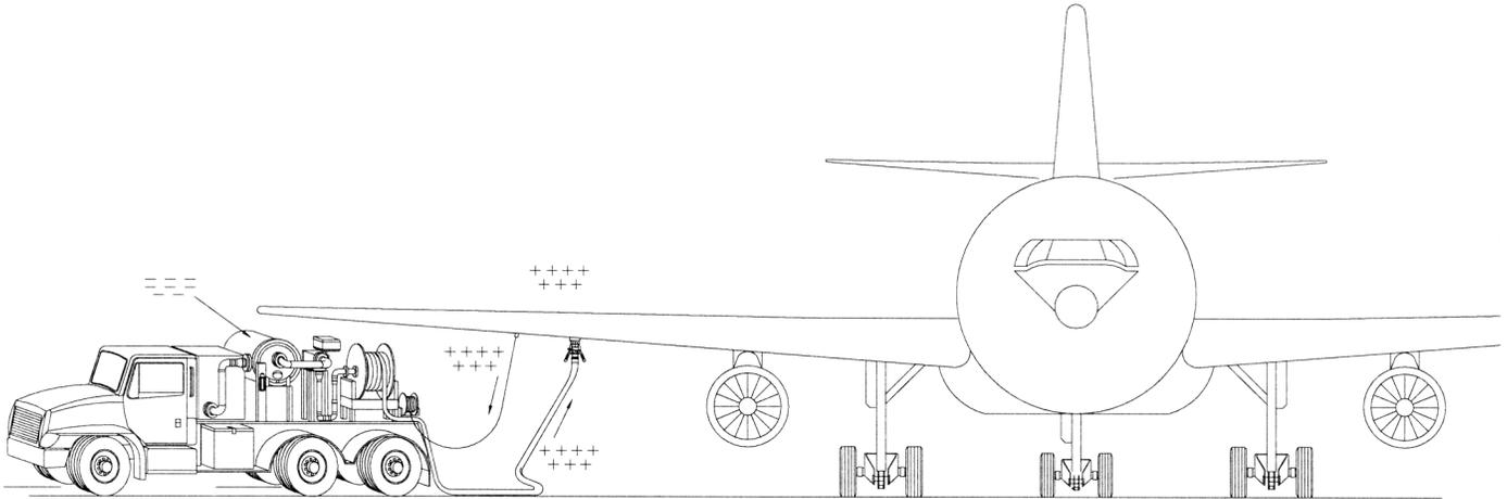
The practice in the USA has been to bond and ground but recent tests have proven that if the aircraft and the truck are bonded, a grounding wire carries no charge at all. This is why NFPA 407 no longer specifies grounding for safety during aircraft fueling.
