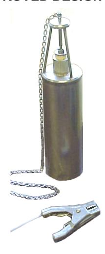
The unique model GTP-9021 was developed specifically to fit through the small gauging found on U.S. Air Force bases where level gauging electric cables are also present. It was important that there be no tangling of our sampler with those cables and that those cables and that those cables not be damaged. Therefore, the outside diameter is only 3.1 in (79 mm).
