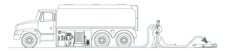
Now walk to the hose reel and lift the hose up high, over your shoulder. Walk toward the nozzle, allowing the hose to slide over your shoulder. This is called "walking the hose". This allows fuel in the hose to empty into the bucket/tub through the strainer, flushing the debris back into the strainer.
