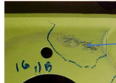
Corrosion of Aircraft Fuel Tank
