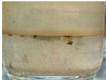
Emulsification at fuel water interface - Microscopic water droplets become suspended in fuel
