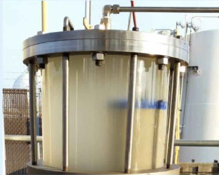
Example of dispersed water haze in fuel
