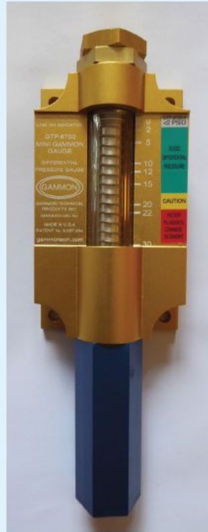
Figure 6: Example of piston-type gauge with quantitative scale for low flow rate/low pressure applications
