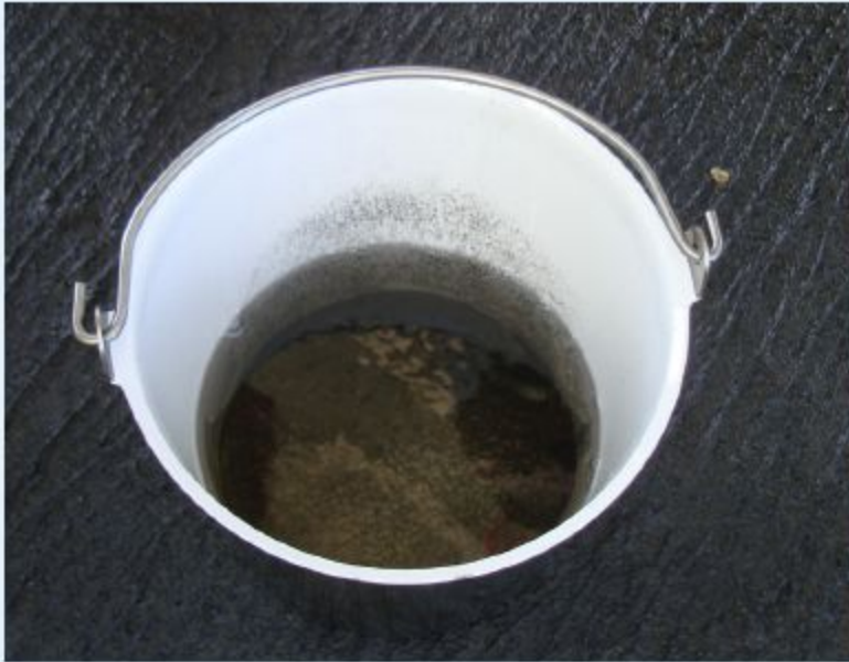
Example of fuel sample containing dirt
